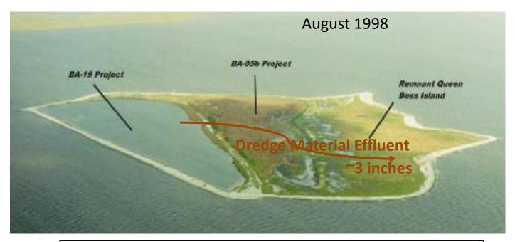
Shell Dike Elevation = 5.22 ft NGVD29 Fill Elevation = 3.72 ft NGVD29 Target Marsh Elevation = 1.22 ft NGVD29 Marsh Elevation 3 yrs Post = 0.79 ft NGVD29, -0.43 ft
