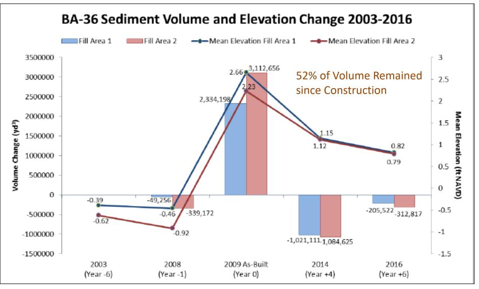
Based on a series of elevation surveys either conducted in or transformed to Geoid 12A
